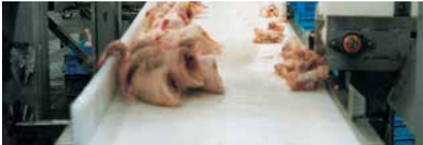
Chicken deboning line with 2015 mattop chain
