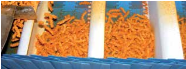
Infeed of inclined conveyor with 2010 isr6
