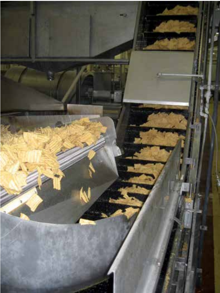
Inclined conveyor for chips ftr2015 mattop chain
