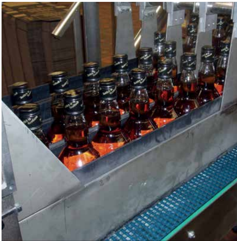
Conveyor with 500 belt.
